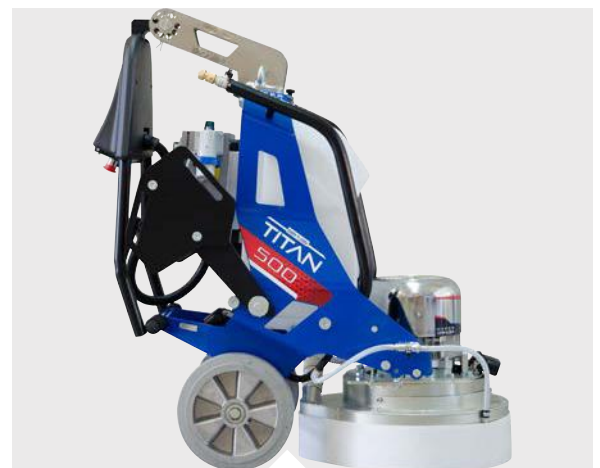
Re-adjustable handle up to 90°.
